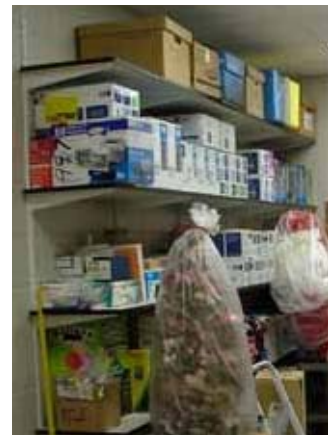
Above are POOR storage practices: storing loose objects on shelf; using top shelf for heavy storage boxes.
